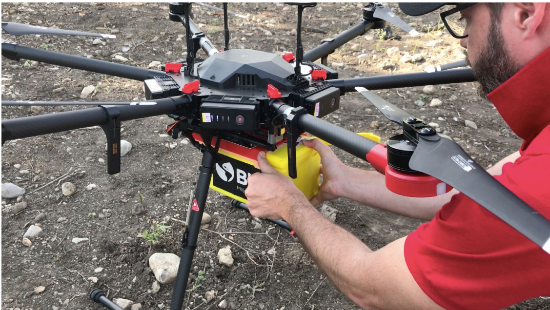
Removing the medical cargo from the M600 drone after landing at a remote clinic in the mountains
