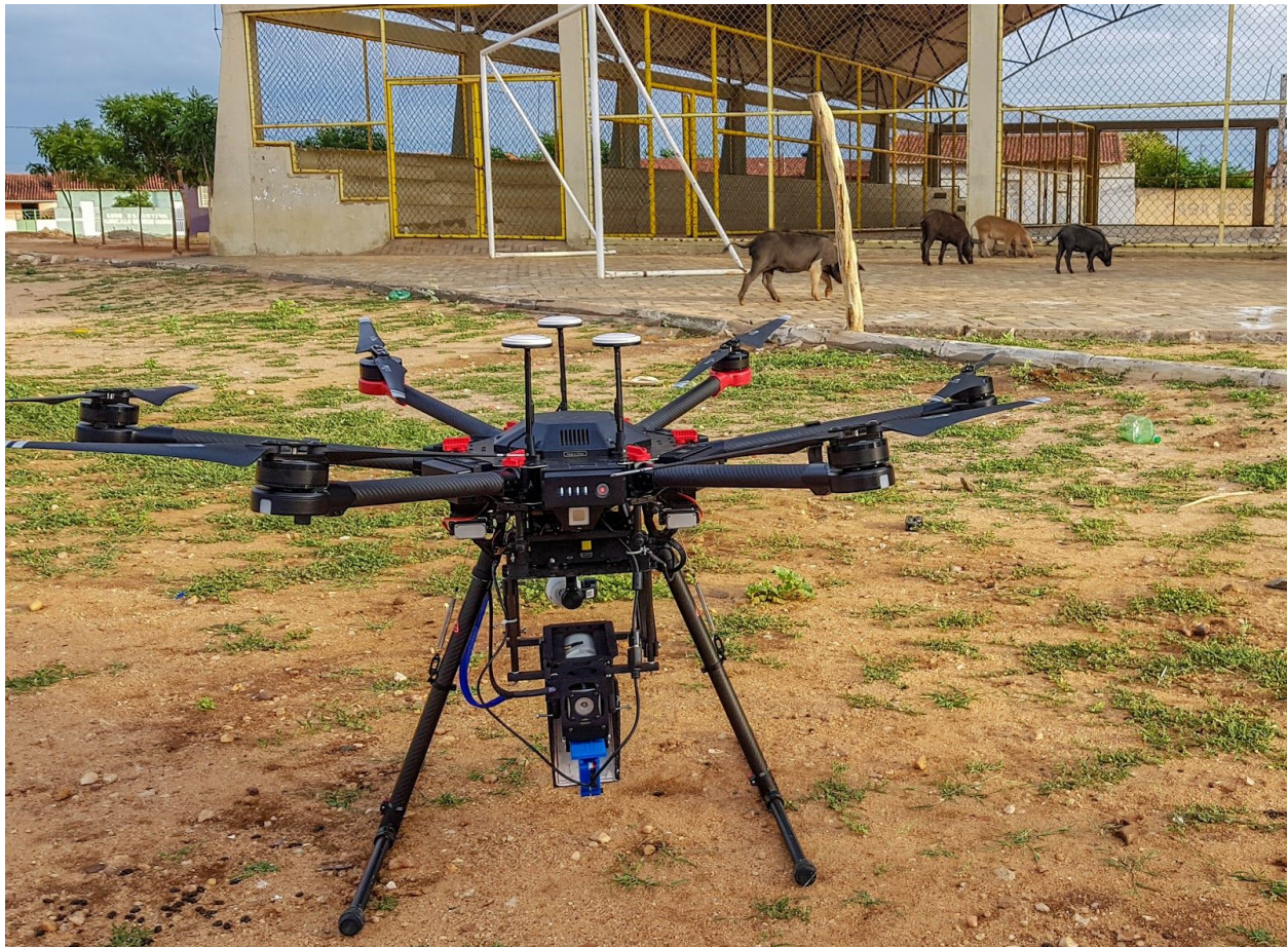
Figure: The Aerial Mosquito Release Mechanism, mounted underneath a drone and waiting for a canister of mosquitoes before a mosquito release flight in Brazil
