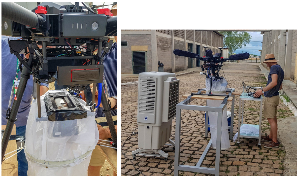
Figure: A net is built around the outlet of the mechanism (left). A flight is then simulated with airflow created by a big fan (right), and all mosquitoes are recaptured.
