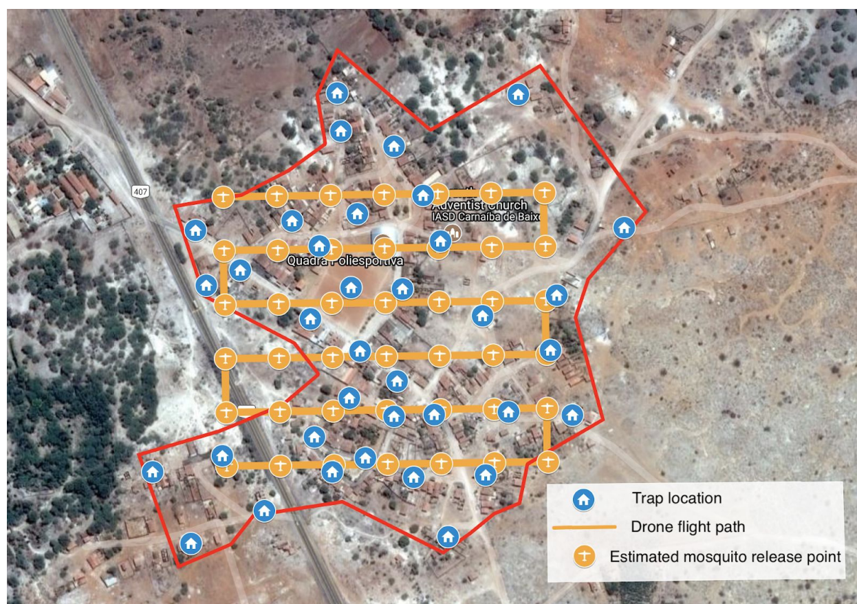
Figure: Flight path of the drone with estimated release points during the homogeneity tests, overlaid on trap locations.
