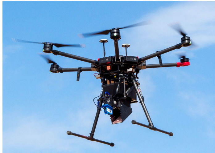
Figure: The fully-assembled aerial mosquito release mechanism attached to a DJI M600 drone
