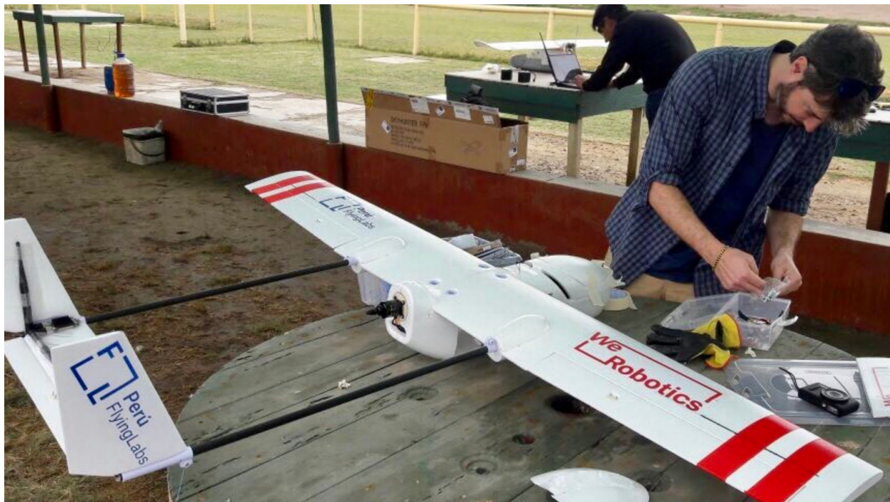
Photo: Assembling and field testing the Amelia cargo delivery drone outside of Lima
