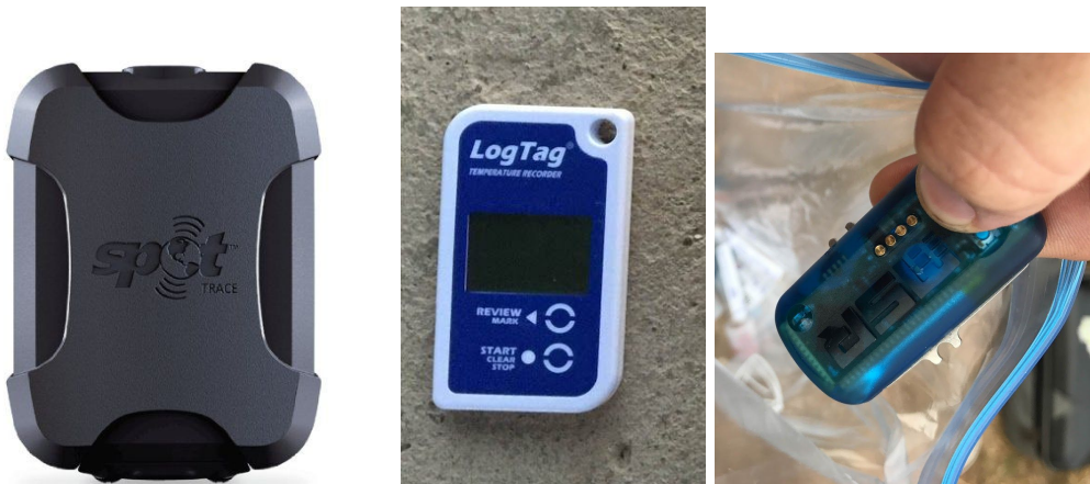
Figure: From left to right, a SPOT satellite tracker, a LogTag temperature sensor and a MSR acceleration sensor.
