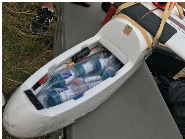
Figure: a plastic bag full of test vials, fit loosely within a Frankie-type drone.
