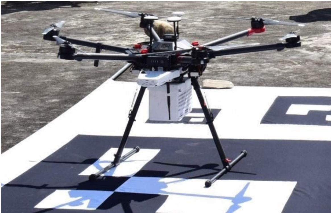
Figure 3.2: The DJI Matrice 600 drone customized as a medical cargo delivery drone for DrOTS.
