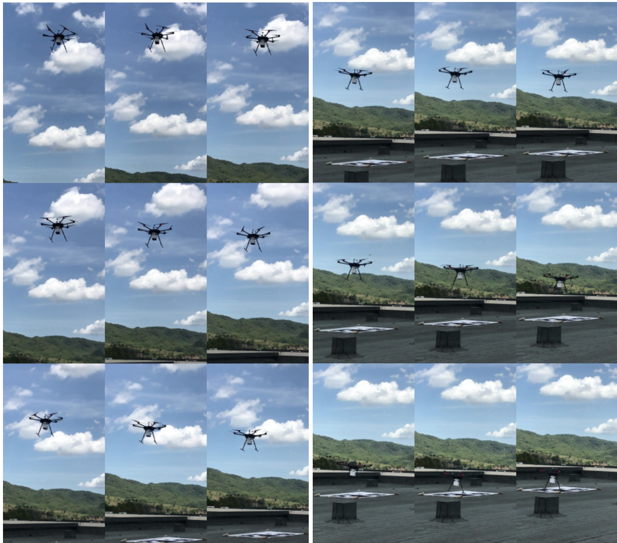
Photo sequence of a fully autonomous precision landing approach in Bohechio.
